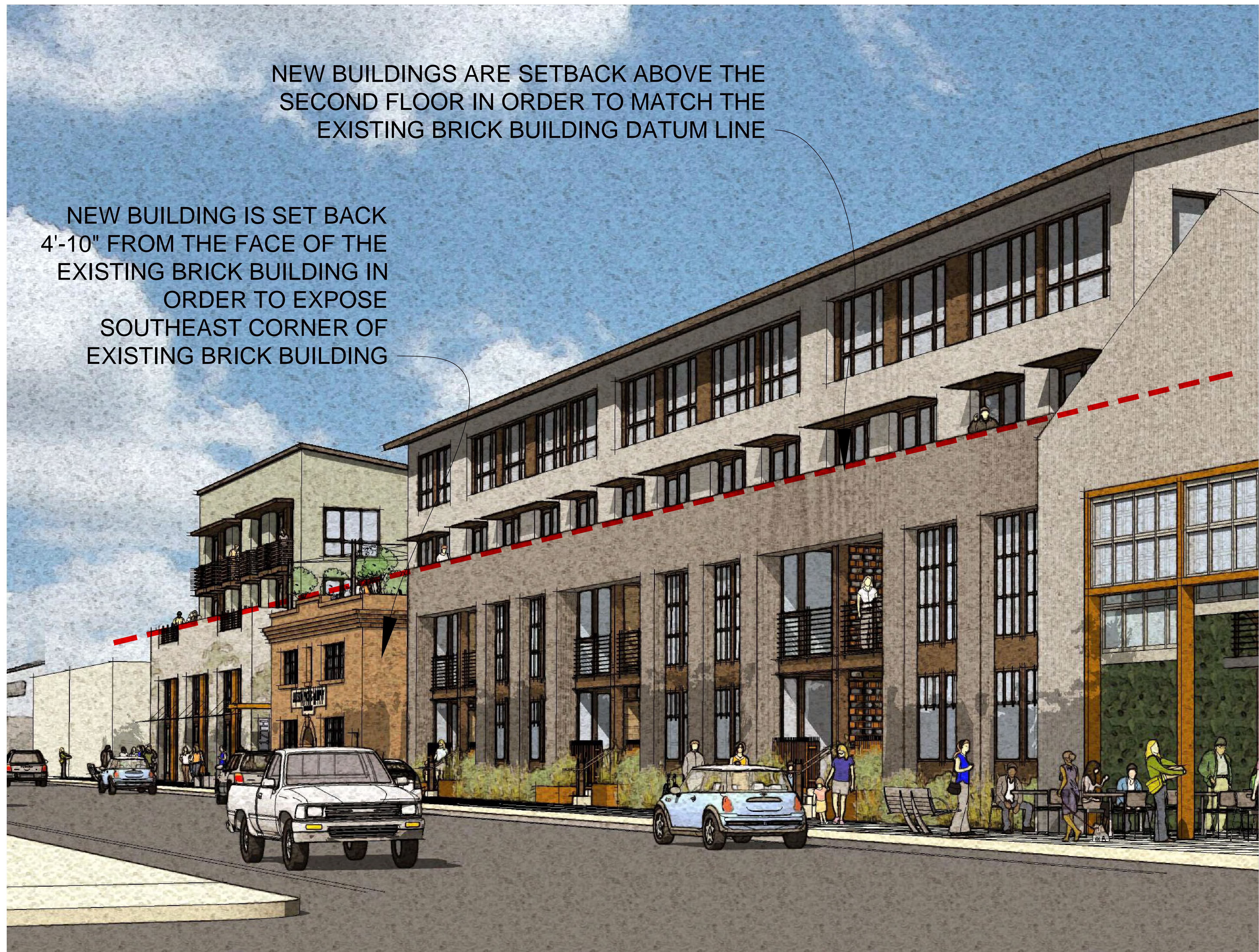
VIEW FROM 17TH STREET LOOKING EAST
